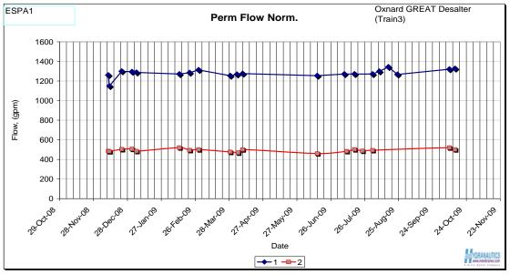
Figure 9: Stable Normalized Permeate Flow over 1 year of operation
