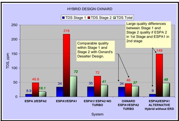
**Figure 8:** Water Quality Improves for Oxnard's 2<sup>nd</sup> stage using turbo boost
