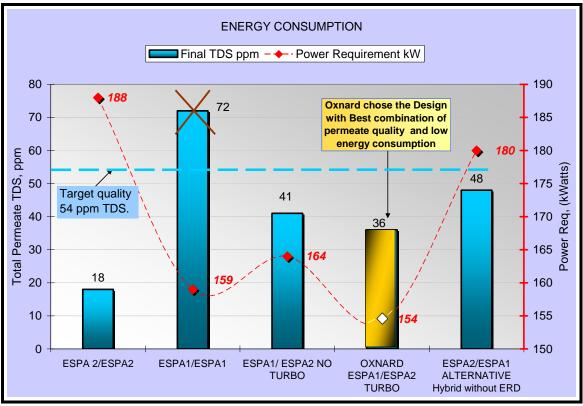
Figure 6: Energy Consumption and Permeate Quality of Different RO Designs using Combinations of Membranes and ERD
