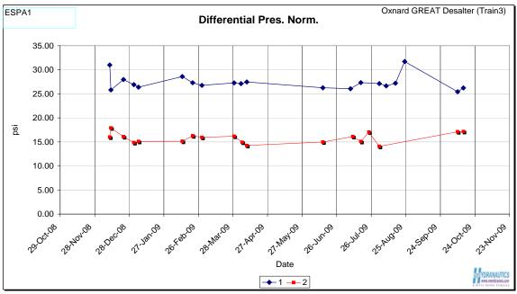
Figure 10: Differential Pressures of Oxnard Desalter Stage 1 and 2
