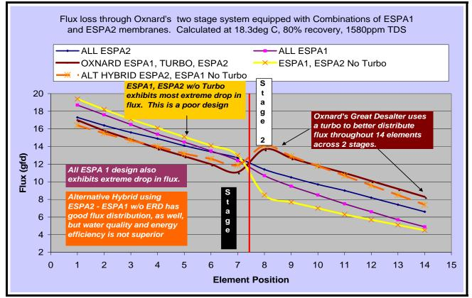
Figure 7: Flux loss in a 2-Stage System with Various Membrane Configurations
